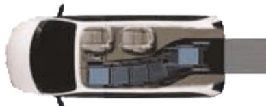
This design places the wheelchair occupant all the way to the front of the vehicle next to the driver without having to move from the wheelchair. This design gives you the freedom to virtually position the wheelchair and yourself anywhere in the vehicle.
